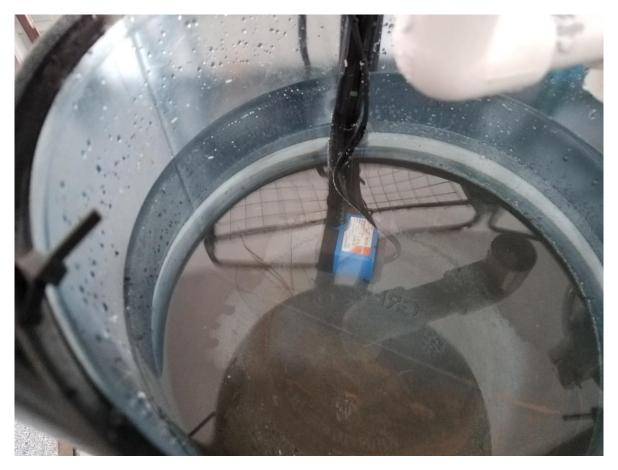
The pump goes into the bottom of your water reservoir and the top of your hose goes into the top so it pours onto the media. You'll need to find a way to secure the top of the pipe so it's doesn't move when the water goes through it and you have a flooded home.
