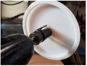
What I do to prebvent this is once the inner drill had slightly penetrated the plastic I then set the drill in reverse and drill the 1" hole in "reverse".
