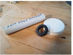
I used a 4" PVC pipe end cap, drilled the hole, inserted the grommet and pipe and siliconed it to the bottom of the top segment as the drain. (pic on left above) The bell-siphon could then rest on top of it. (pic below)
