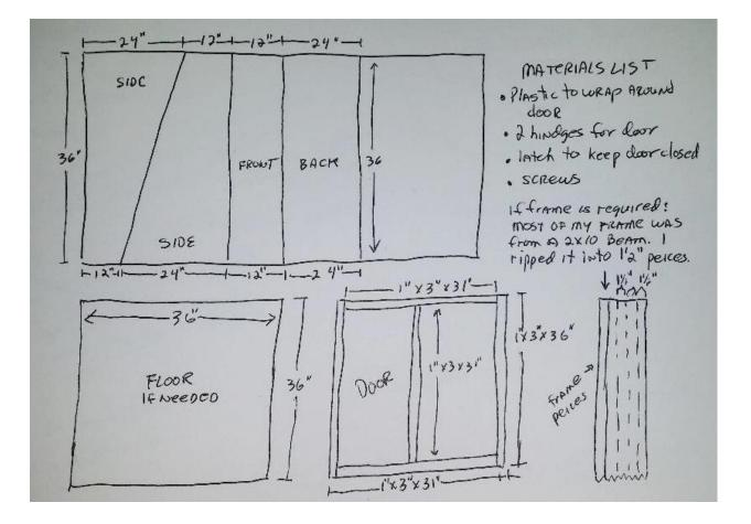
I used 1/4" plywood because I had lots of it for flooring in my garage. Since it's so thin I used 1 1/2" pine to frame it for strength. I ripped the pieces from a 2"x10" beam I had left over from another project. You can use 1"x3" pine strapping in if you like.
